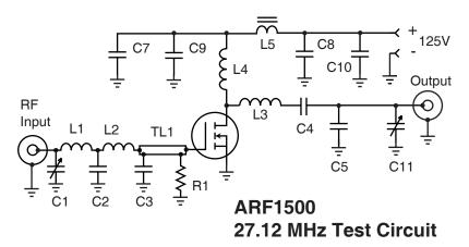
C1,C11 ARCO 465 50-450pF mica trimmer C2 1500pF ATC 700B
